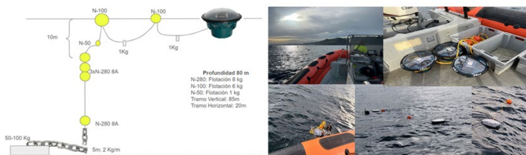
Figure 10 (Left) Wet connection system between each buoy and the main line of the longline (Right) Deployment of Zunibal acoustic sensors attached to the main longline in the experimental area.
