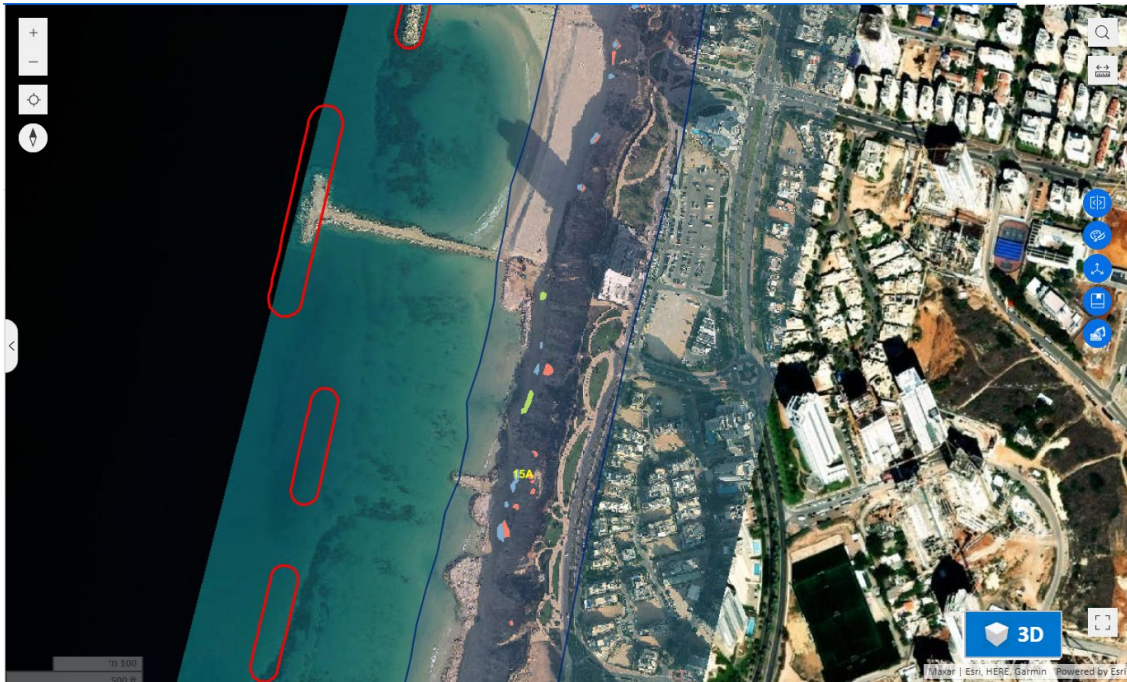
Figure 3 Map of showing location of cliff collapse events in 2023. Location of cliff collapse events (red) since 2010; debris accumulated at the base of the cliff (blue); areas where debris was washed out to sea (green). (data source: MCCP – Mediterranean Coastal Cliffs Preservation).
