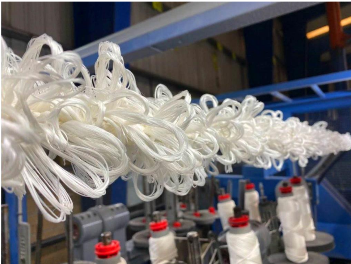
Picture 2: Shows the production of the first prototype of the new rope type (BIOGEARS). From https://www.azti.es/en/biogears-biodegradable-ropes/
